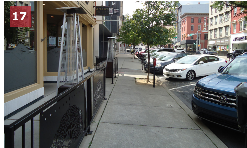
Outdoor seating and street tree/parking meters may partially obstruct pedestrian access route.
