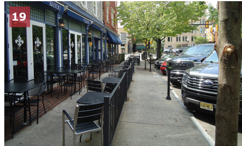
Pedestrian access route is limited by outdoor dining and parking meters/street tree.
