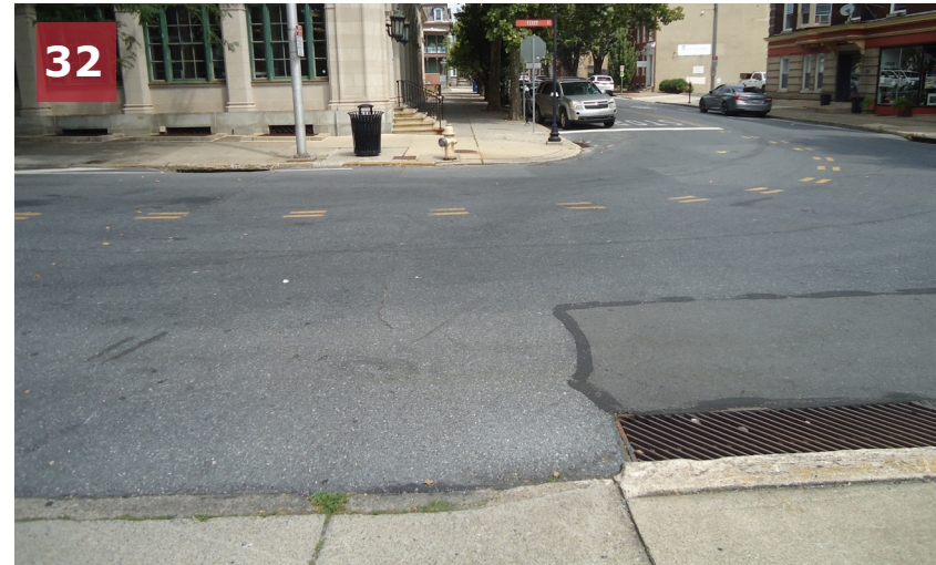
Missing curb ramps at the intersection of Second Street & Ferry Street (two corners).
