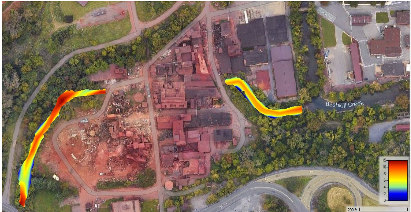
Maximum flow velocity (ft/s; at water pool) of 100-year flood for the pre-development condition.
