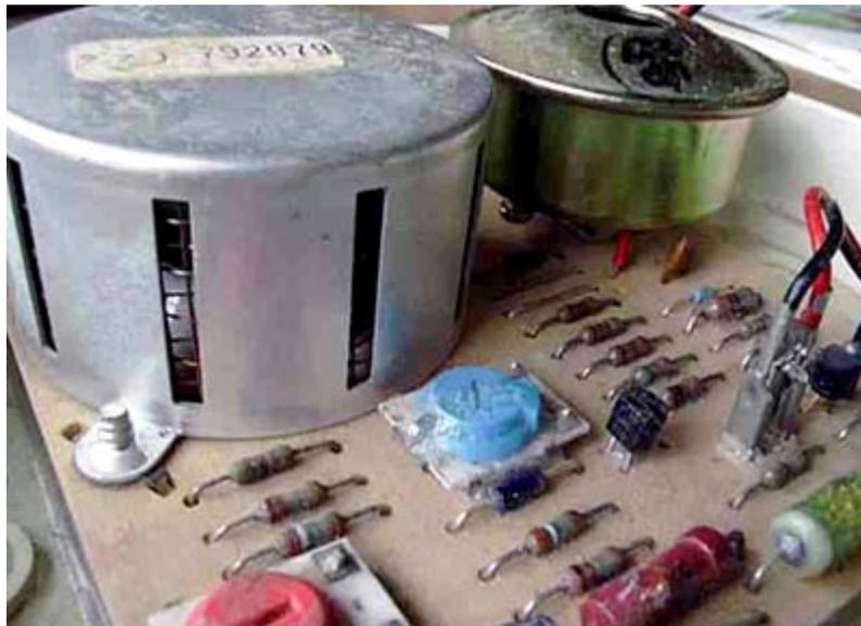
Underneath the can is a ceramic holder that contains the positive plate of the ionization chamber. Under that plate is the ionization source, **WHICH YOU WANT TO BE SURE NOT TO DISTURB**.
